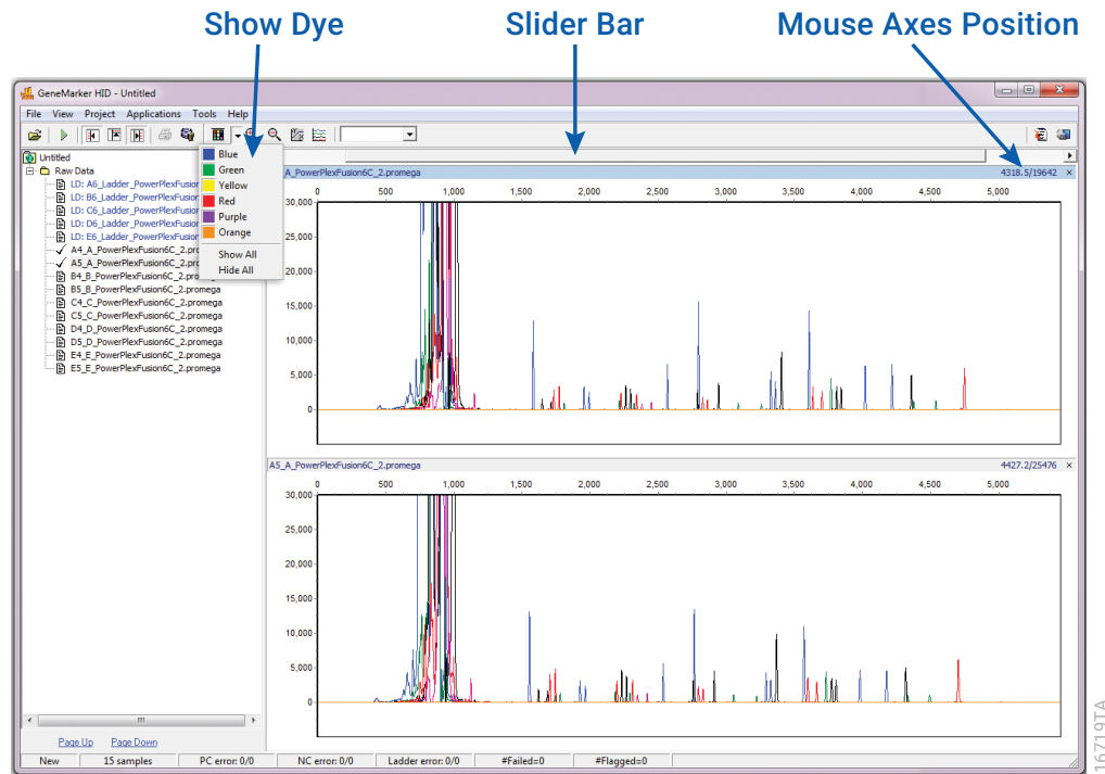
Figure 55. Raw data in the 'Main Analysis' window.
