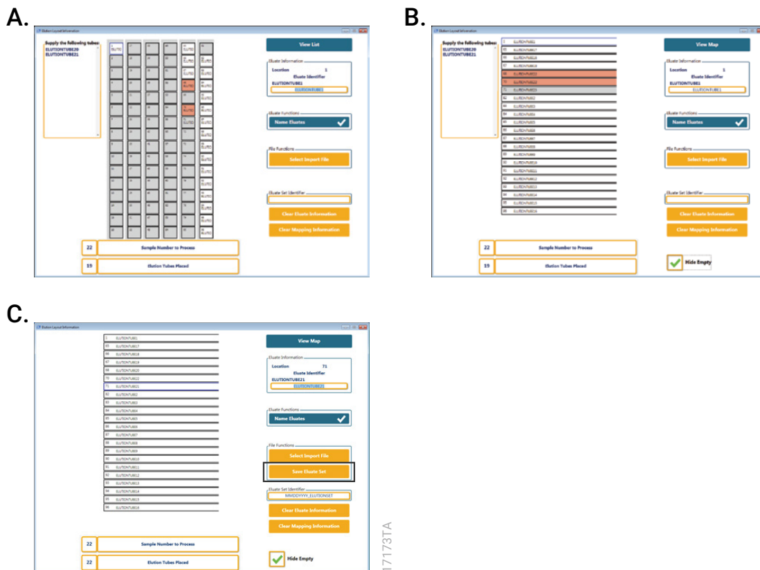
Figure 15. Modifying Information in the ‘Elution Layout Information’ windows and Save Eluate Set. Panel A. Map View. Select the View List button to display a list of elution tube identifiers. Panel B. List View. The salmon-colored tube positions and the “Supply the following tubes:” box (upper left corner) indicate that the imported list contained two positions with the same elution tube identifier and the list did not contain elution tube identifiers that map to each sample identifier, respectively. Both issues must be resolved before the method can proceed. Position 71 contains an elution tube identifier; however, its gray color indicates the identifier is not mapped to any sample identifier. The tube at position 71 will not be used. Checking the “Hide Empty” box collapses the empty elution tube positions (i.e., positions containing no identifier). Panel C. Modifying Imported Elution Tube Identifier Information. The salmon-colored entries at positions 68 and 70 (Panel B) indicate that duplicate identifiers are detected. Highlight position 68, select the Eluate Identifier input box, manually provide one of the unique and required identifiers and press the Tab key. The listing of identifiers in the “Supply the following tubes:” box (Panel B) indicates additional elution tubes are needed on the worktable. Highlight position 71, choose the “Eluate Identifier” input box, manually correct the incorrect elution tube identifier and use the Tab key. To remove all elution tube identifier information or the information that maps the sample identifiers to the elution tube identifiers, select the Clear Eluate Information button or the Clear Mapping Information button, respectively. When the required information for the elution tubes has been added and no replicate identifiers are detected, the Save Eluate Set button will be displayed. Select the Save Eluate Set button.
