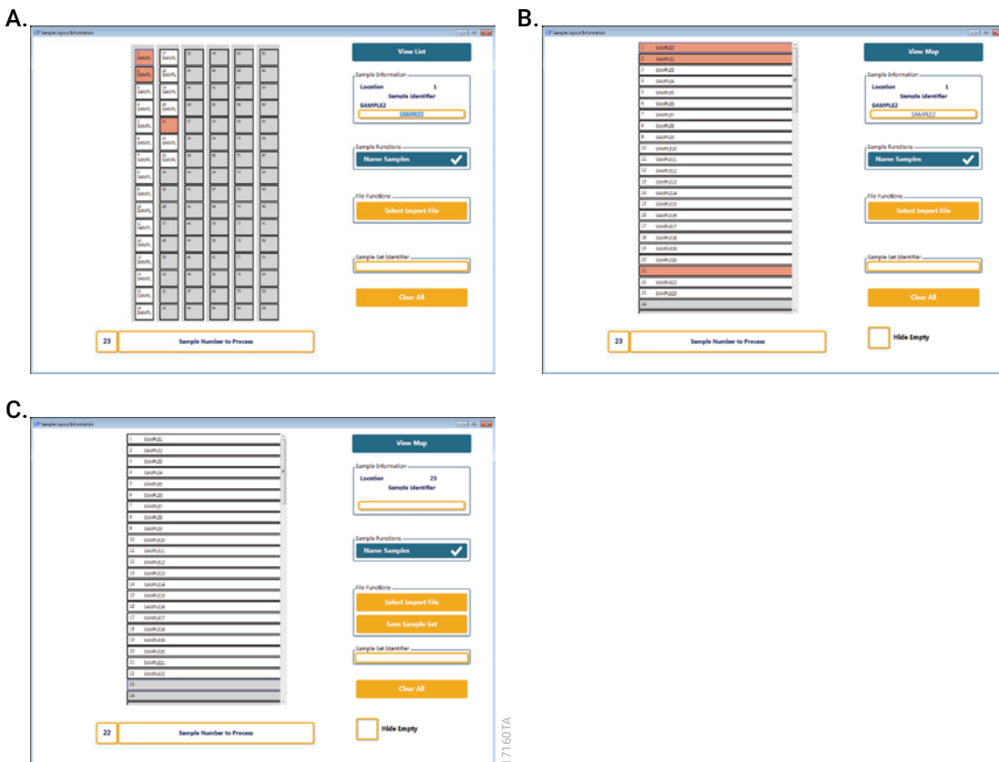
Figure 5. Modifying Information in the ‘Sample Layout Information’ window. Panel A. Map View. Choose the Select Import File button (initial window shown in Figure 4, Panel A) navigate to and load an import list; the results of the actions are shown. Salmon-colored positions indicate issues with the imported sample identifier list that must be addressed before the method may continue. Select the View List/View Map toggle button to display the sample information in list format. Panel B. List View. Modifying Imported Sample Identifier Information. The salmon-colored entries at positions 1 and 2 indicate replicate sample identifiers are detected. Highlight position 1, select the “Sample Identifier” input box, manually provide a unique sample identifier and use the Tab key. The salmon-colored entry at position 21 indicates the import file contained no sample identifier information. As there are sample identifiers supplied for positions 22 and 23, manually supply a unique sample identifier for position 21. Highlight position 21, select the “Sample Identifier” input box, provide a unique sample identifier and press the Tab key. Finally, to delete sample identifier from a position, highlight the position (e.g., position 23), select the “Sample Identifier” input box, manually delete the sample identifier and press the Tab key. Panel C. List View. The Save Sample Set button is visible when all the sample status issues are resolved.
