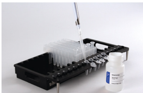
Figure 2. Setup and configuration in the deck tray(s). Elution Buffer is added to the Elution Tubes as shown. Plungers are in well #8 of the cartridge.
