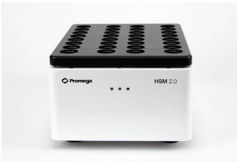
Figure 4. Front of the HSM 2.0 Instrument showing LED informational lights. Green—power on/off; Yellow—user prompt; Red—error.
