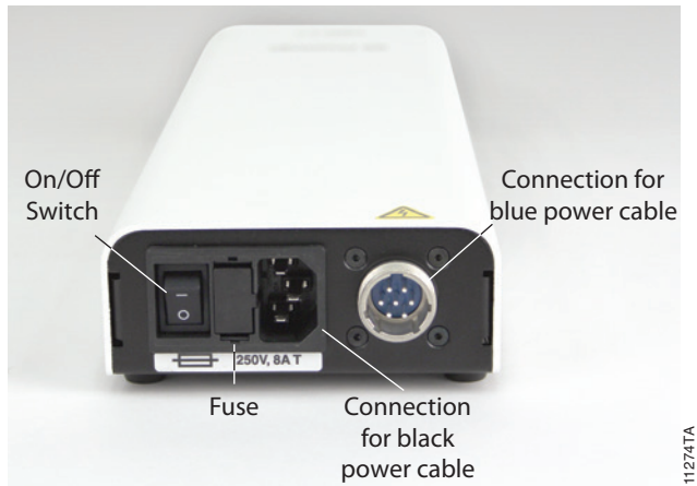
Figure 6 Rear of the Power Supply showing the main power switch, fuse, and power connections.
